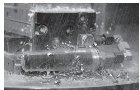
10 pressure sensors with radio transmission
